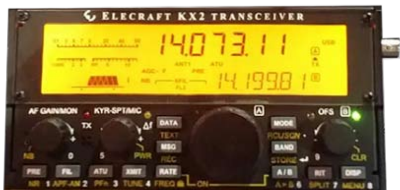
Elecraft KX2 QRP transceiver with optional built-in tuner
