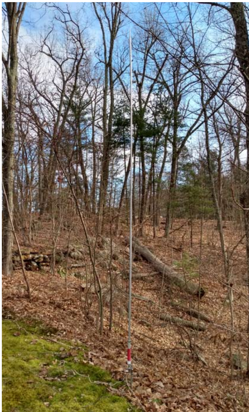
Vertical Antenna with Coil & Counterpoises
