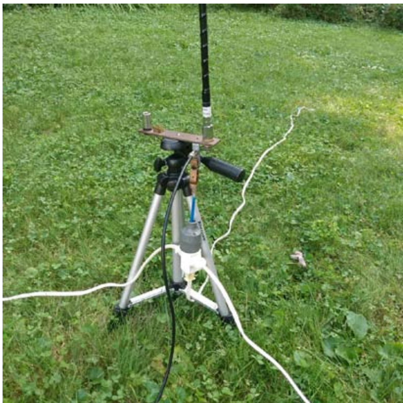
Radial Kit Deployed with hamstick antenna and tripod mount
