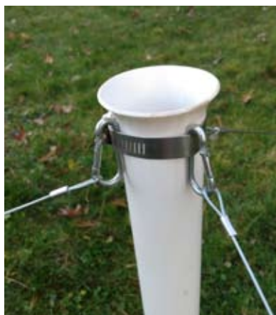
Snap Links at Top of Spike secured with hose clamp
