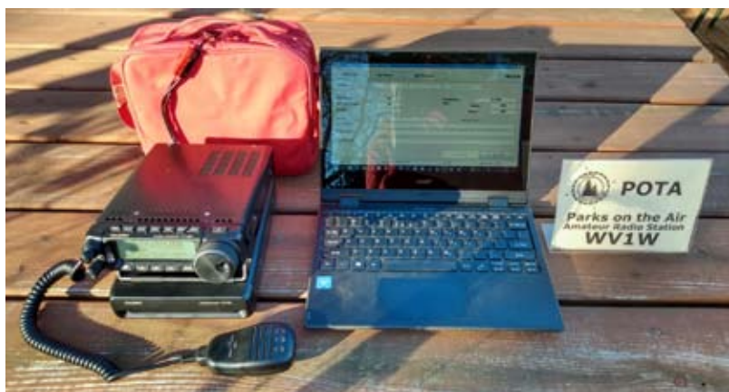
Yaesu FT-891 with FC-50 tuner fits conveniently under radio
