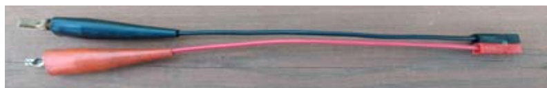
Battery Clips to Powerpoles® Adapter for running a rig directly from the car's battery
