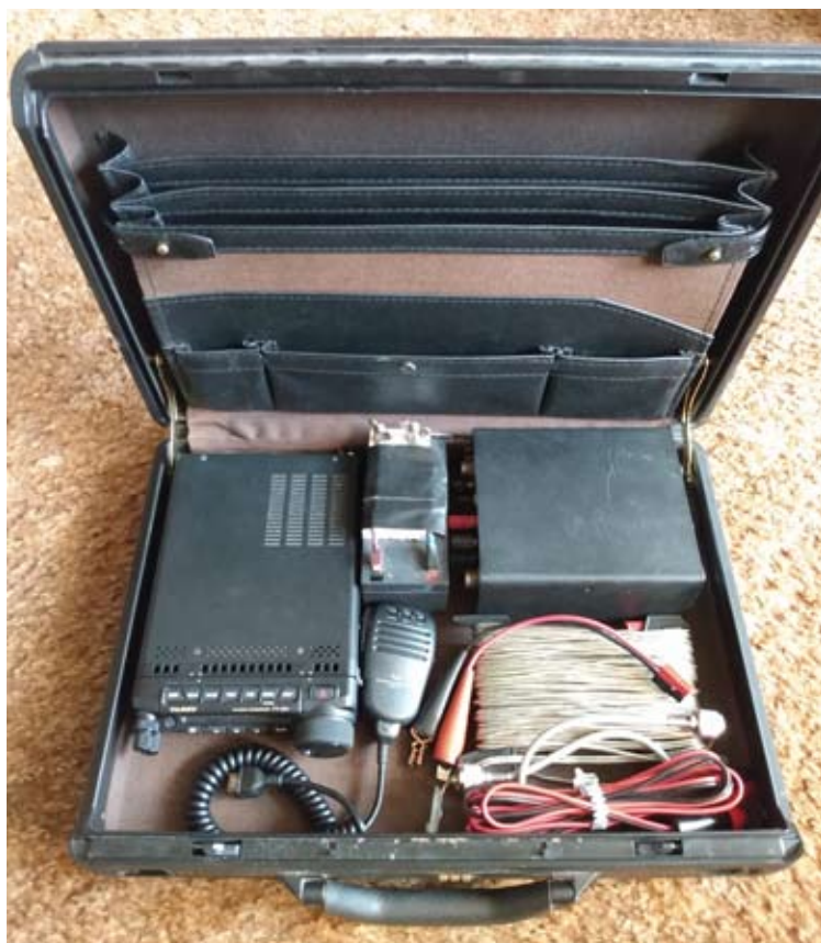
Complete Station Packed in a Briefcase rig, tuner, battery, mic, and antenna
