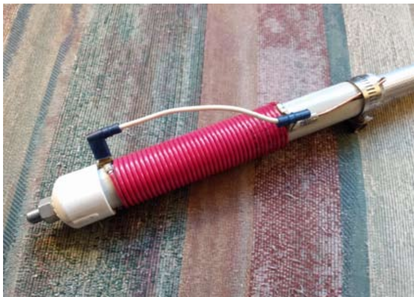
40m Loading Coil with easily removable jumper for 20m
