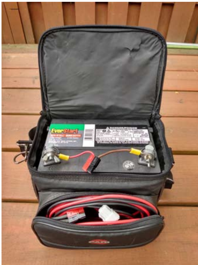
U1 Battery in Camera Bag with rig power cable in front pouch
