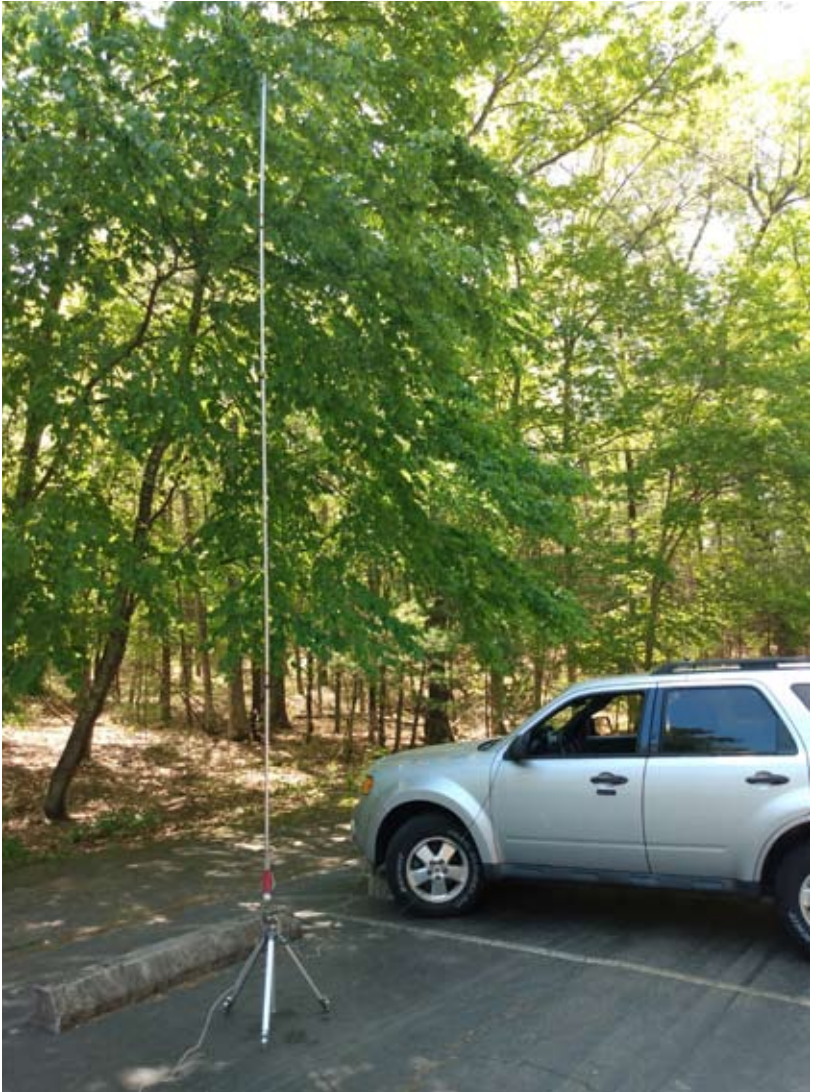
Vertical on Tripod with Counterpoise Wires
